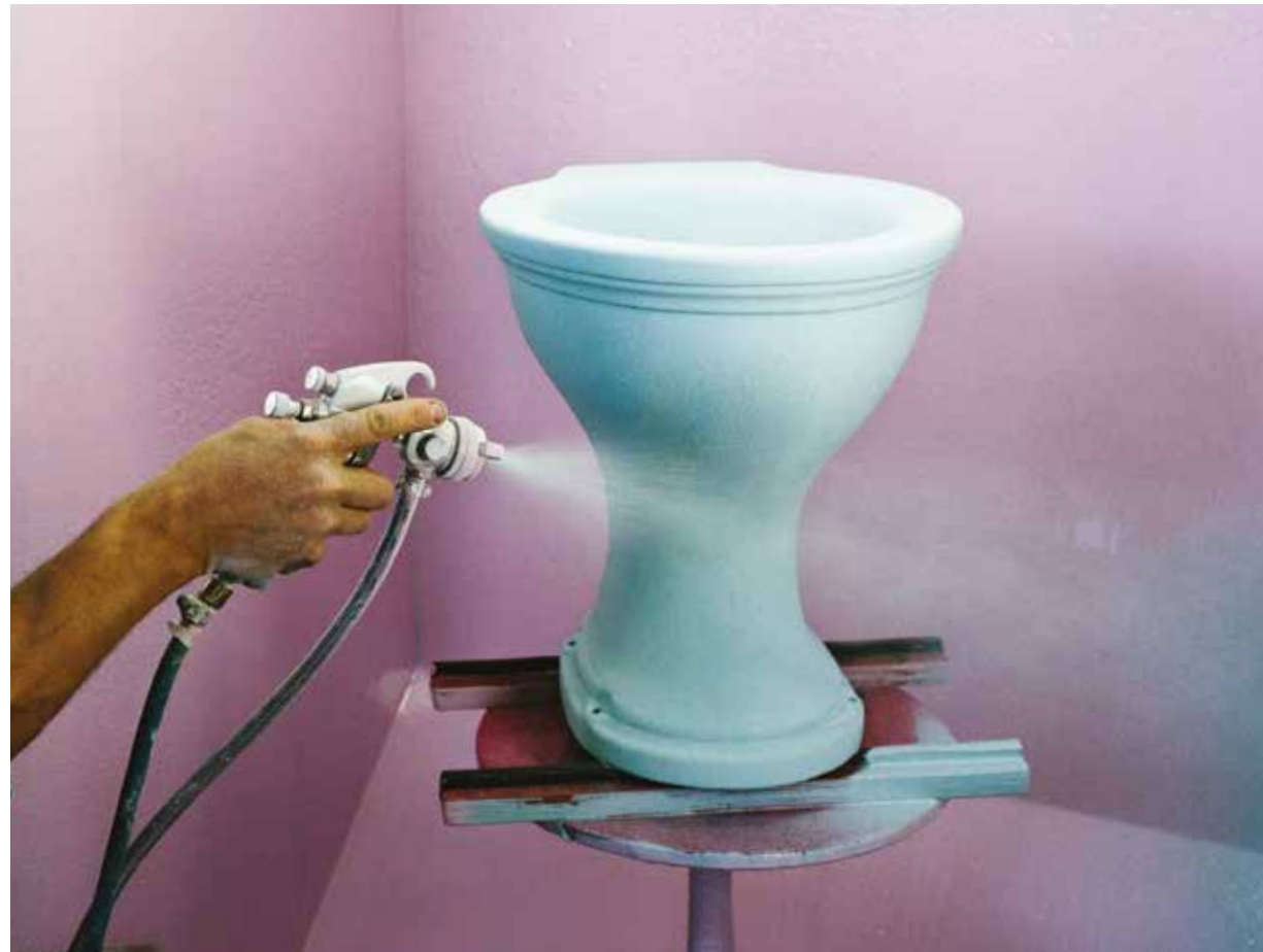
HAND SPRAYING THE GLAZE PRIOR TO FIRING.
