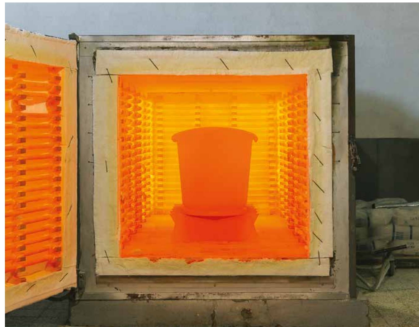
EACH BATH IS HEATED TO 960°C SEVERAL TIMES DURING THE ENAMELING PROCESS.
