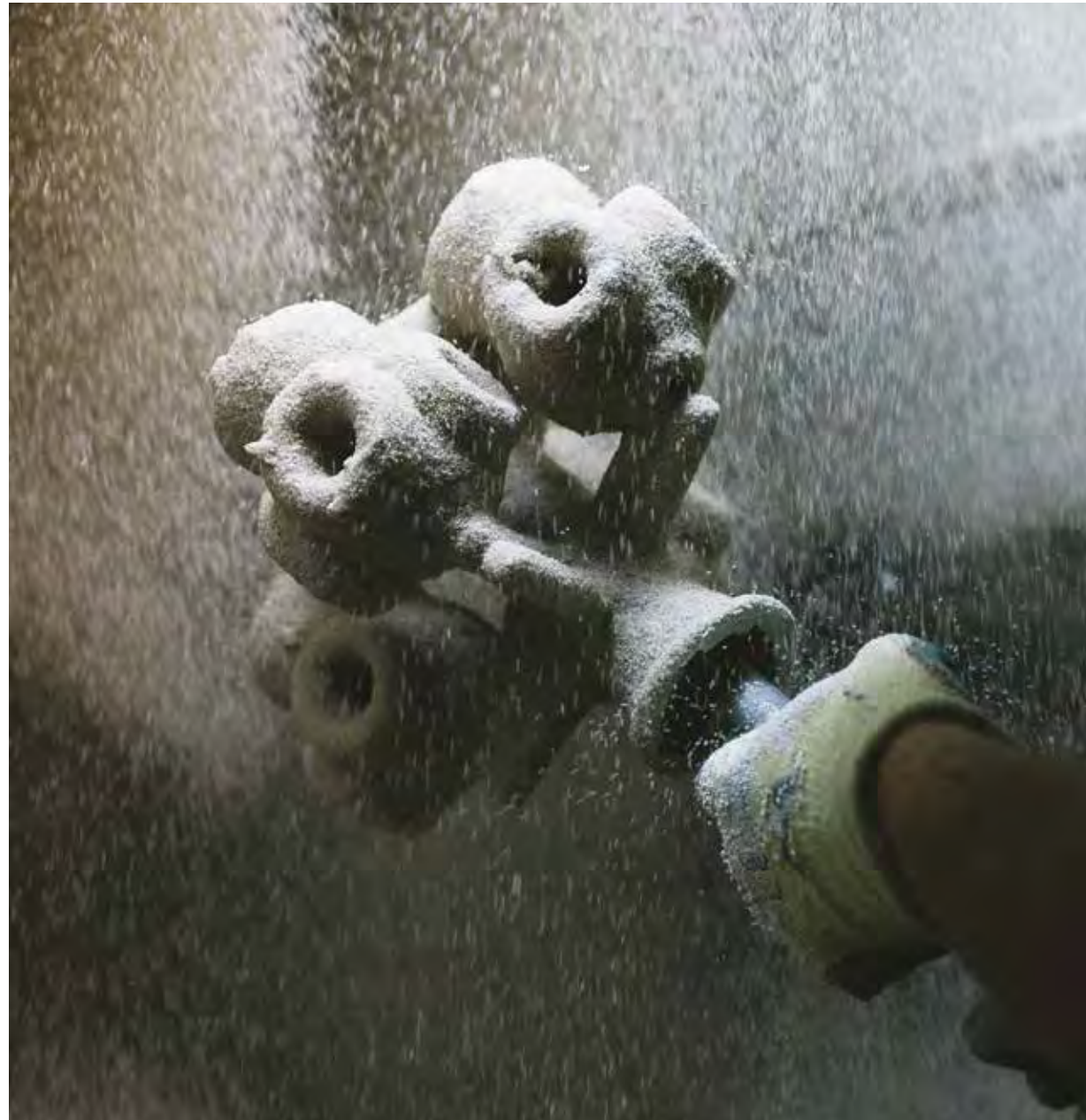
A COCOON IS BUILT UP TO COAT THE WAX MODEL.
