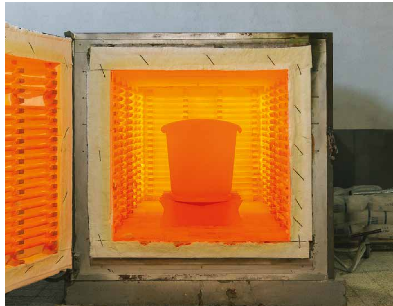
EACH BATH IS HEATED TO 960°C SEVERAL TIMES DURING THE ENAMELLING PROCESS.
